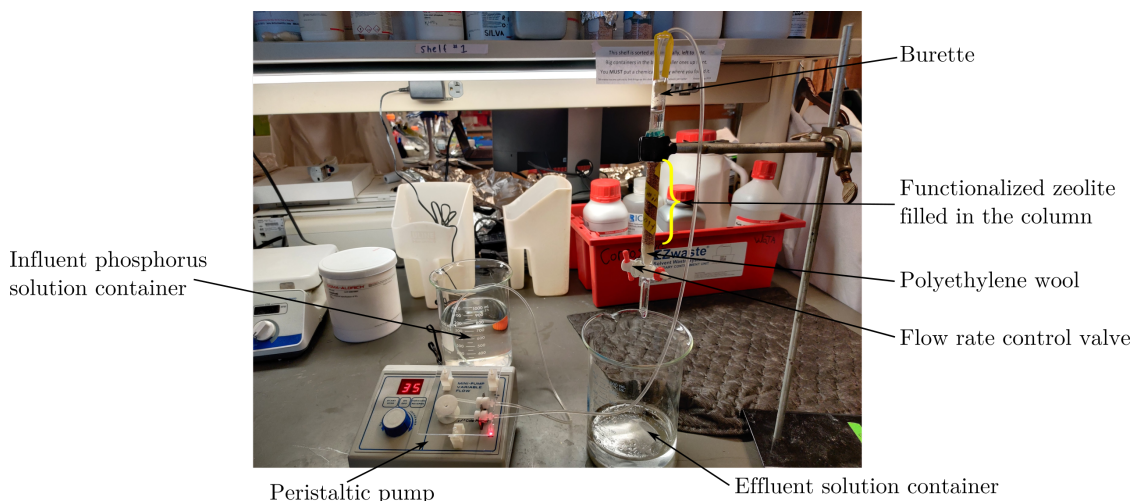
Figure 5.3: The experimental setup of the column-flow experiment.
